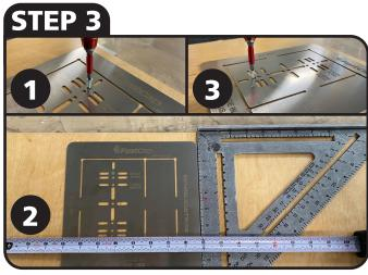
SCREW JIG TO PART WITH SCREW MARK. USE SQUARE OR TAPE MEASURE TO ALIGN JIG. ADD 2ND SCREW TO HOLD JIG IN PLACE.
