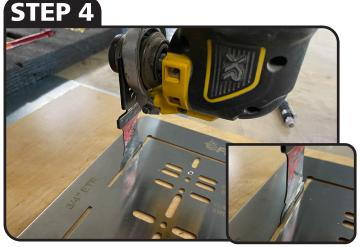
USING AN OSCILLATING SAW, CUT WITH SQUARE BLADE TO THE OUTSIDE EDGE OF JIG.
